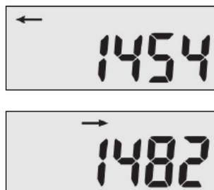
When there is no activity and no counts are made, the LCD display will automatically switch between both directions.
